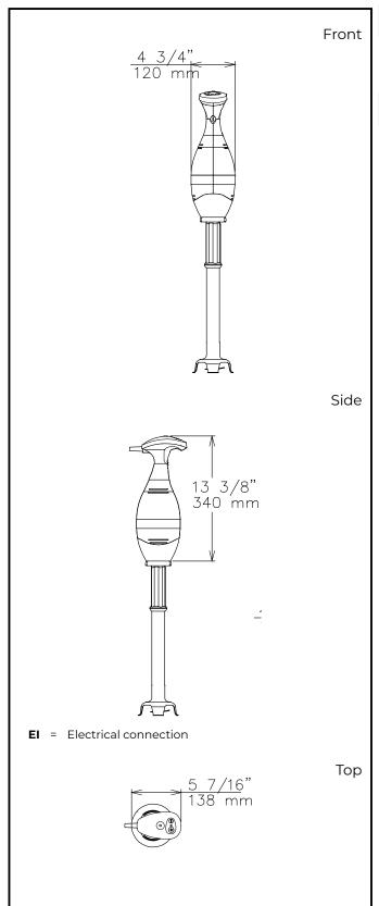
Electric Supply voltage: 110-120 V/1 ph/50/60 Hz **Total Watts:** 0.35 kW Plug type: USA NEMA 5-15P Key Information: External dimensions, Width: 5 7/16" (138 mm) External dimensions, 4 3/4" (120 mm) Depth: External dimensions, 30 1/8" (765 mm) Height: **Shipping width:** 11 7/16" (290 mm) Shipping depth: 27 3/16" (690 mm) Shipping height: 7 1/16" (180 mm) **Shipping weight:** 12 lbs (5.3 kg)
